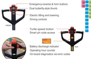
• The function of driving with tiller in the vertical position helps with operations in confined areas without sacrificing safety
