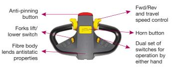
Operator never has to leave the handle during application making operations stable and safe
