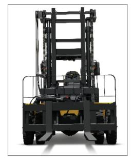
Upright section of the mast is reinforced with heavy tie bars. The 4 lateral thrust carriage rollers resist deflection caused due to off-centre loading
