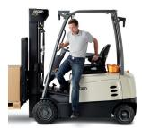
Operators easily get on and off the truck due to the low step height, spacious floorboard and sculpted seat deck. The contoured overhead guard provides superior head clearance.
