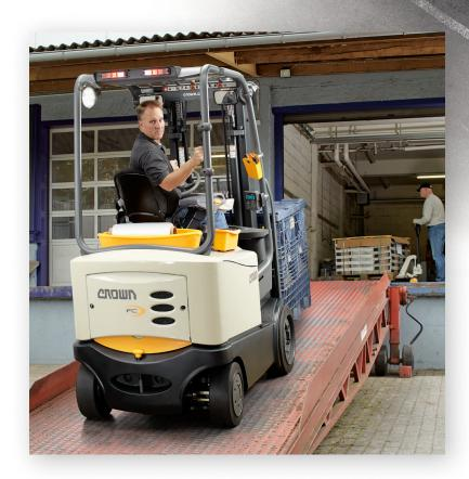
Travel and corner speed control automatically limits travel speeds during movement and turns, based on load weight, lift height and steering angle. 1462
